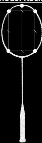
Equal amount of lead tape (white, filled circles) added to 5 lightweight (72g) base frames
