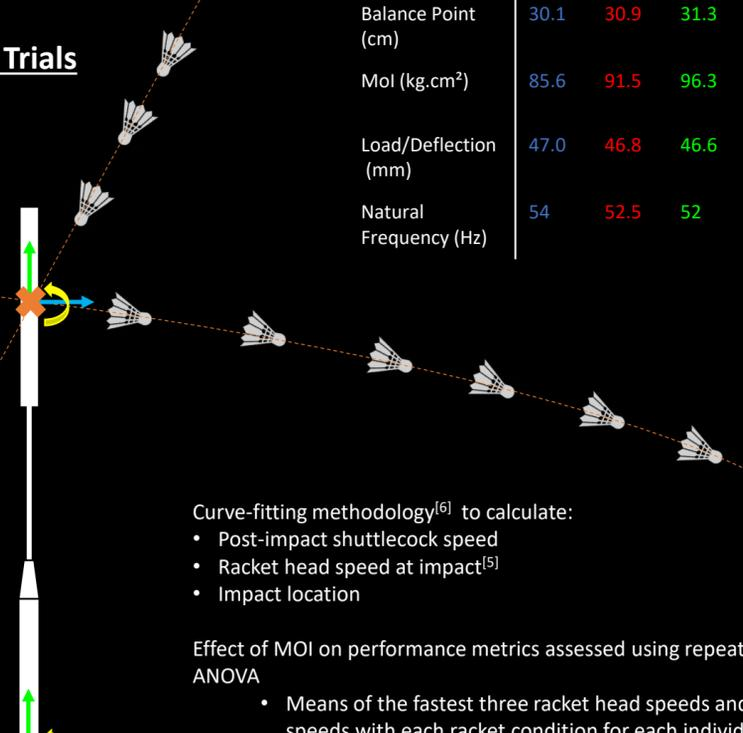
Deflection defined by the transverse angle between handle and frame segments, using Euler angles
